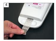
Once removed, try to touch only the "handle" end of the cartridge (curved edges) to place the cartridge into the reader.
