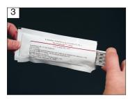
If refrigerated, allow cartridge (in pouch) and sample to warm to room temperature before proceeding. Remove cartridge from pouch by touching the edges of the cartridge.
