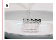
Holding the pipette straight up and down at the bottom of the sample well can force some sample into the channel early and disrupt the reagent mixing stations. Avoid any technique which is prone to splash out or bubbles.
