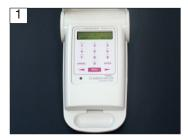
Press the MENU key on the PTS™ to turn the reader on. The reader begins a "System Self Test" and heats to 37°C in approximately 5 minutes.
