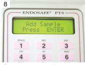
Once the reader displays "Add Sample Press ENTER" the assay is ready to be initiated. Press "Enter". After assay is complete, results appear on screen. Data can be printed or downloaded to computer.
