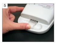
Insert cartridge firmly into the slot at the front of the reader with the sample reservoirs facing up.
