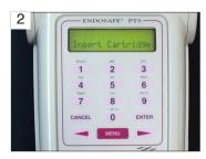
Once the reader reaches 37°C the reader display will change from "System Self Test" to "Insert Cartridge".
