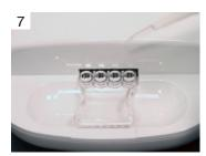
When prompted by the on board software to add the sample, hold the pipette so that the tip is at an angle and not completely at the bottom of the sample reservoir.
