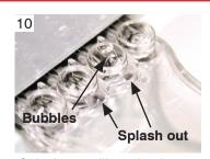
Splash out will render the volume inaccurate which can lead to invalid test results. Bubbles can cause false onset times due to the disturbance of light transmittance and can interfere with reconstitution of reagents within the cartridge.
